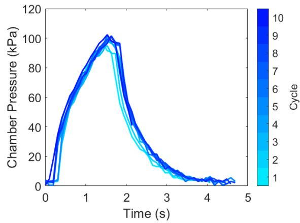
Figure S1: Consistency of the soft ring oscillator. Pressure was measured at one node of the pneumatic circuit for 10 cycles and overlapped to show the consistency in the pressure oscillations in this component of the pneumatic circuit.
