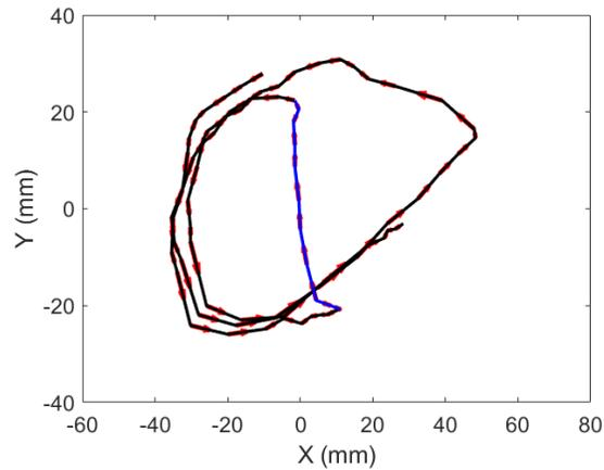
Figure S2: Motion of the foot of the robot when the pressure in the pneumatic controller is perturbed. The position of the foot followed a cyclical trajectory during a normal oscillatory cycle (colored black). After the pneumatic circuit controlling the leg was temporarily perturbed by reducing the input pressure to atmosphere, the position of the foot deviated from the cyclical trajectory (colored blue). When this leak was sealed, the leg returned back to the normal oscillatory movement.
