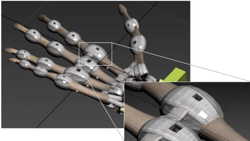
**Fig. S1. Hand CAD model showing the finger ligament designs.** Hand CAD model showing the finger joint design, with the inset picture showing how the softer ligament material has square cut outs to allow the support material to be removed from the joint area after printing.
