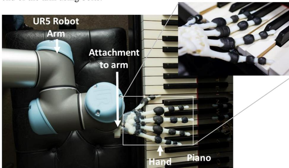
**Fig. S2. Full experimental setup.** Showing the UR5 Arm. The attachment of the hand to the arm and the 3D printed hand. The UR5 arm is placed such that it is perpendicular to the environment, which is in this case the piano.
