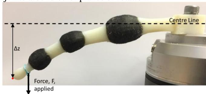
**Fig. S4. Experimental method to determine the compliance of a single finger.** The three joints of the finger are used, with the finger fixed at a given orientation. A force is applied with the displacement of the finger tip in the direction of the force measured.
