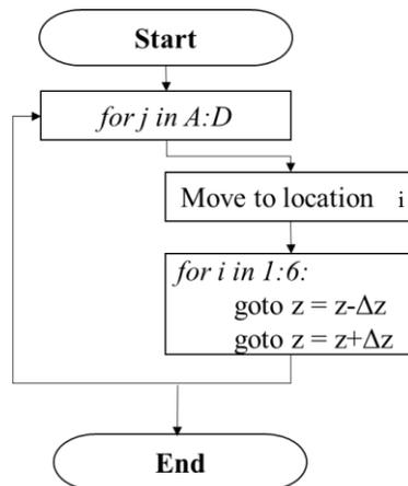
Fig. S6. Flow chart of the motion planning required for playing *Toccata*. Repeated note playing at the four different locations.
