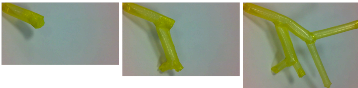
Fig. S4. Extension of a soft robot body with preset pattern of branching. Multiple branches can be preprogrammed at time of manufacture.
