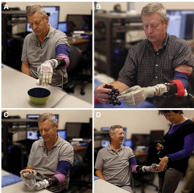
**Fig. 6. Sensory feedback supports ADLs.** The participant performed several one- and two-handed ADLs while using the sensorized prosthesis, including moving an egg (A), picking grapes (B), texting on his phone (C), and shaking hands with his wife (D).
