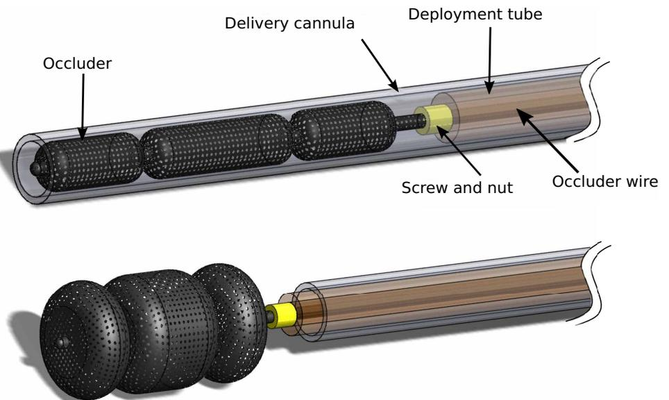
**Fig. 6. Occluder deployment system.** The occluder, attached to a wire via a screw connection, is preloaded inside a flexible polymer delivery cannula. The delivery cannula is inserted through the lumen of the catheter into the paravalvular leak. A polymer deployment tube is used to push the occluder out of the delivery cannula. Once positioned, the occluder is released by unscrewing the wire.
