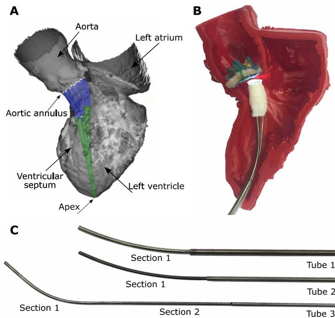
**Fig. 4. Algorithmic robotic catheter design.** (A) Computer model of optimized design composed of three tubes shown in adult left ventricle. Robot enters heart through apex and is depicted at 12 locations on the aortic annulus. (B) Fabricated catheter with haptic vision sensor shown inside 3D printed model of heart shown in (A). (C) Disassembled catheter showing its three precurved superelastic tubes. Tube parameters are given in Table 1.
