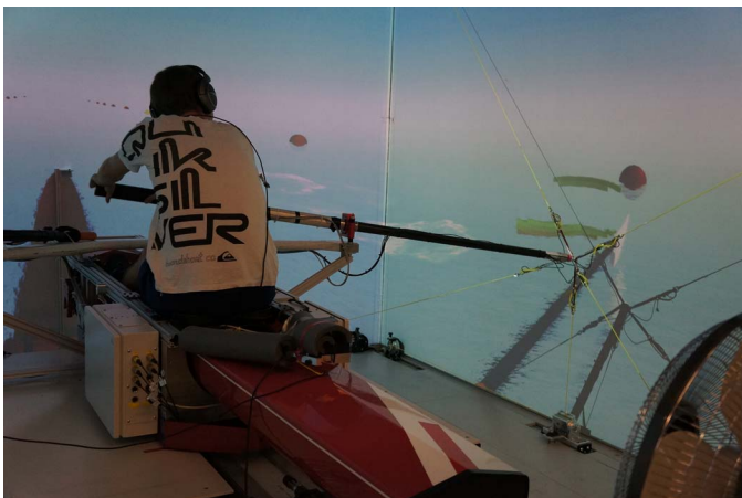
Fig. 3. Coauthor demonstrating the rowing simulator. Participants were seated in a real rowing boat placed in a CAVE. The participant's task was to perform a predefined rowing oar movement only with arms and upper body (roll seat was strapped back to prevent the rower from bending the legs). When the virtually prolonged oar was moved through the virtual water, the rower saw, heard, and felt realistic oar-water interactions. In addition to rendering haptic oar-water interactions, the tendon-based parallel robot was used to haptically guide the participant if the related feedback design was selected. The current photo shows visual feedback during the drive phase (green and red dots drawn right above and below the blade).
