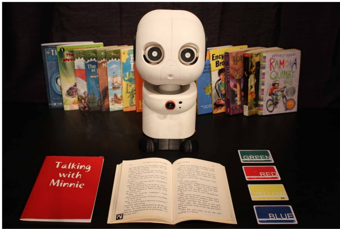
Fig. 1. Minnie and study materials. The learning-companion robot and the study materials, including the Talking with Minnie book, RFID cards, and books augmented with AprilTags. The robot's camera, the red circle on the upper torso, is used to read AprilTags and to track the child's face. A microphone, visible to the right of the camera, is used for audio-recording sessions, and an RFID reader, below the camera, not visible, is used to recognize cards for simple commands.
