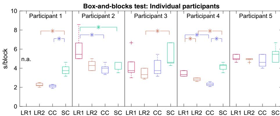
**Fig. 2. Results from box-and-blocks test.** The reported outcome measure is the average time per block. Performances of LR-based control on two different days without retraining (LR1 and LR2) and two conventional control strategies, CC and SC, are shown separately for each participant (one panel each). LR was robust across sessions, and its performance was similar to or better than the conventional control systems in the second day, although only one DOF was needed. n.a., not applicable.
