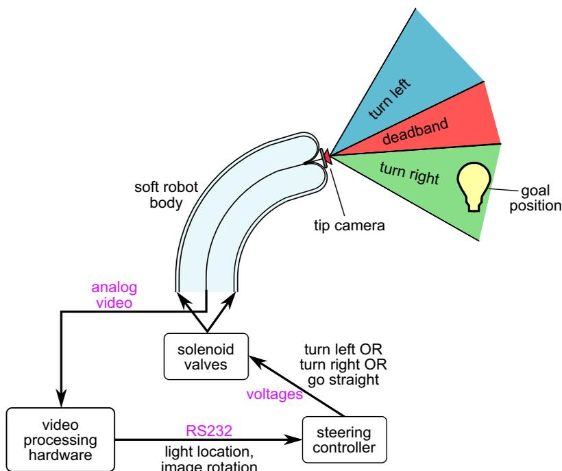
**Fig. 6. Overview of active steering control system.** Hardware components and a physical depiction of the steering task are shown. Electrical signal formats are labeled in purple, and their semantic meanings are labeled in black.
