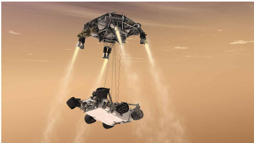
Fig. 4. Mars 2020 rover being deployed by Skycrane (courtesy of JPL/NASA).
