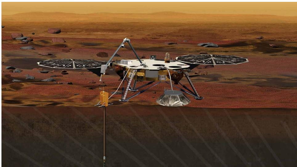
Fig. 3. InSight lander with a robotic instrument deployment arm and a seismic sensor and a heat flow sensor deployed (courtesy of JPL/NASA).
